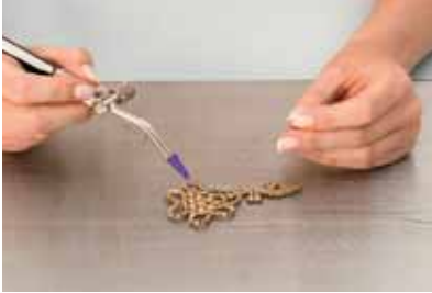
1 Solder the original model.
