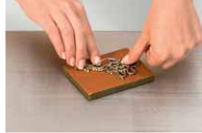
3 Press the original model into a suitable impression material.
