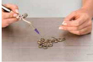
2 Strengthen the rear of the original model with wire.
