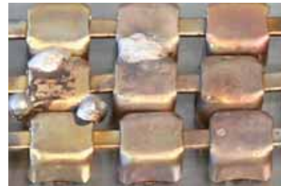
3 Too high temperature
