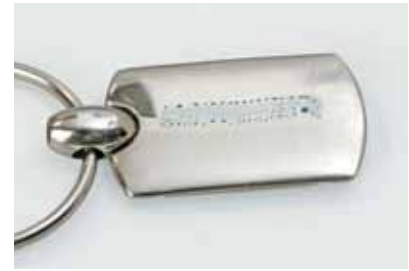
3 If the ink disappears or forms bubbles, the surface is not suitable for applying Ceralun. In this case, the pre-treatment cleaning methods should be checked.
