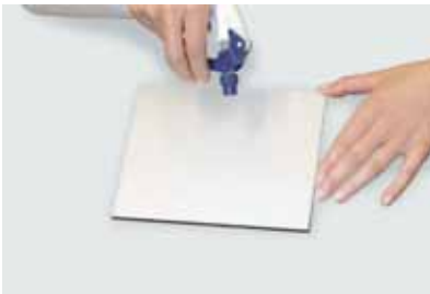
1 Moisten the cleaned surface with soap water.
