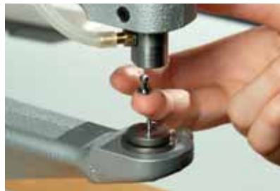
5 Place the lower part in the upper die (crystal pointing upwards).
