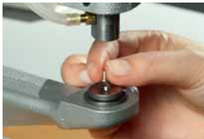
4 Place the lower part of the Crystal Stud in the lower die.
