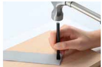
9 Create the buttonhole with a buttonhole punching tool (art. 9040/122).
