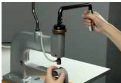
7 Apply the Crystal Stud by closing the handle.
