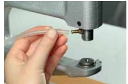
3 Connect the vacuum pump and turn it on.
