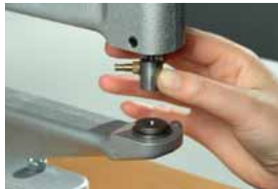
2 Place the tools in the fly press. Make sure that they are sitting straight and firmly.
