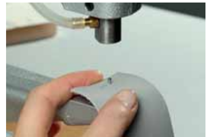
6 Put the carrier material with the pre-punched hole over the lower part.
