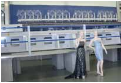
4 Embroidery is carried out automatically using a system like the Laesser Crystal Stone Head (in the photo) or the Tajima Lochrose Embroidery Device.
