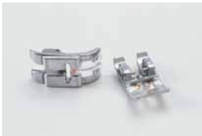
Adapted presser feet/beading feet (e.g. for single-row Plastic Trimmings): standard presser feet, adapted by adding two metal plates.
