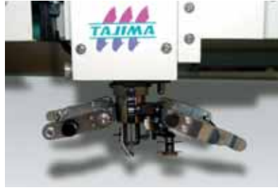
The lock stitch head is ideal for applying single-row Plastic Trimmings.
