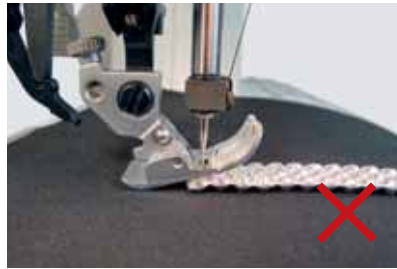
A slanting presser foot can cause problems with the feed of the base material.
