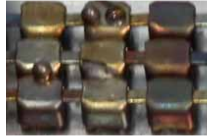
3 Too high temperature
