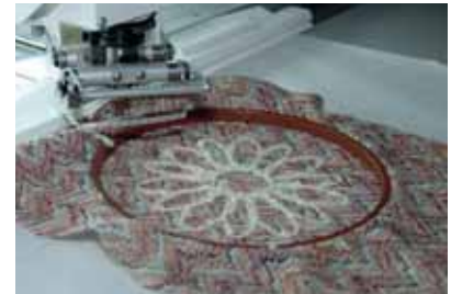
A frame serves to stabilize thin and elastic fabrics during industrial embroidery processes.
