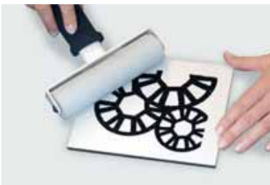
4 After drying, press down firmly on the motif again, e.g. using a rubber roller.
