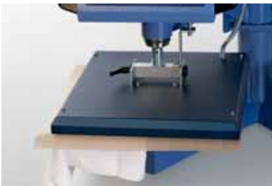
4 After pressure, time and temperature are set, close the heat press.
