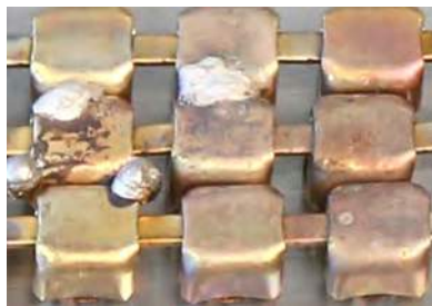
2 Too high temperature
