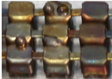
2 Too high temperature
