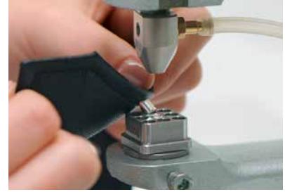
3 Turn the fabric around, place an already applied 3D Stud in one of the linear grid's cavities, crystal side facing down.
