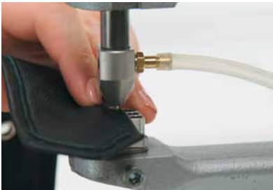
4 Place a Back Part in the upper die and close the handle of the fly press.
