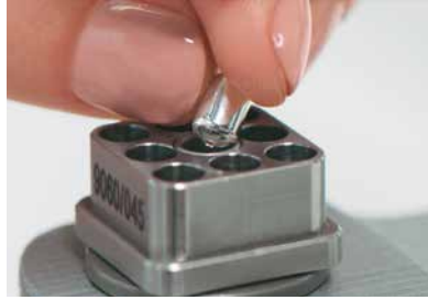
2 Set a 3D Stud, crystal pointing downwards, in the lower die with proper insert (big cavity in the middle of the linear grid).
